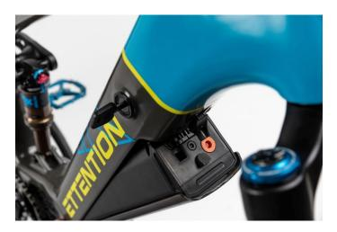
competing formats are considerably less space-efficient. A 36V battery's 10S4P or 10S5P arrangement only manages 63% space utility, a 48V battery's layout (13S3P, 13S4P or 13S5P) reaches no more than 65% – plus, that "high-end" 48V battery leads to a very wide package which conflicts in particular with the requirements of state-of-theart downtube integrated batteries.
